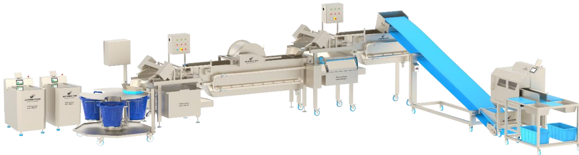
The ACBM in a vegetable processing line for cutting, washing and drying vegetables
